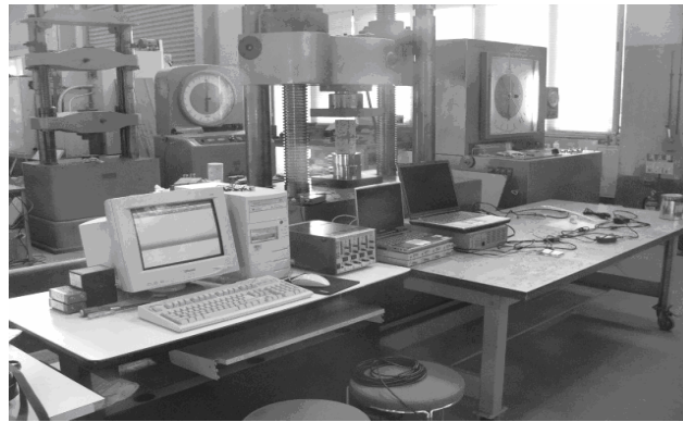
Figure 6. AE measurement in the compression test.
