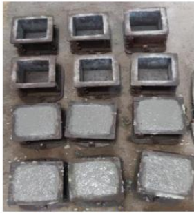
Figure 2. Filling of concrete moulds.
