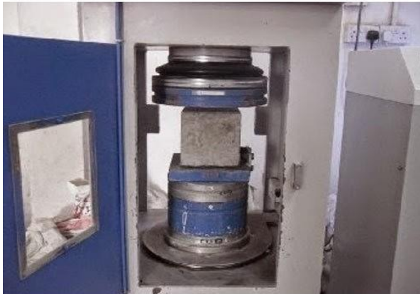
Fig .1 Compression test on cubes
