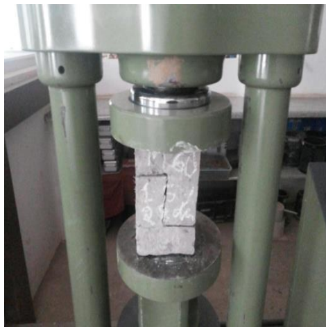
1. Typical Dimensions of Push-off Specimen Used and a Failed Specimen under
