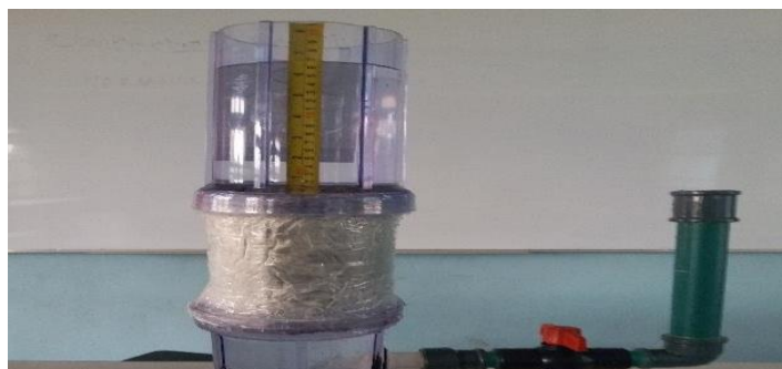
Fig 2: Permeability test of pervious concrete
