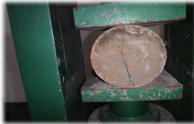
FIG II: Split tensile strength ( f_s = (2W)/(\pi LD) )
