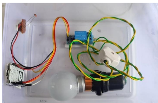
Figure 7: Prototype of the IoT based smart street light system
