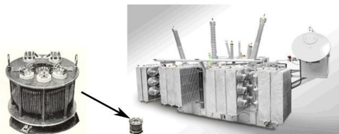
Fig.3 The left side of the pictures shows one of the first core type power transformers, manufactured at the GANZ factory in 1886, rated power was 7.5kW [27]. On the right side the size of this transformer is compared with a modern large power transformer.
