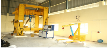
Fig P 6.2.6 Structural Engineering Laboratory (Load Frame of 100 tonnes capacity)
